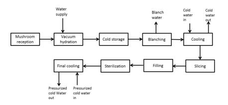
Fig 5.1: Schematic flow diagram of the current production of canned mushrooms
