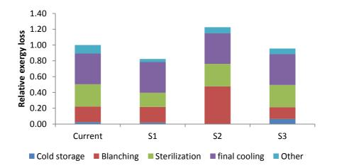
*Figure 5.10: Relative exergy losses of various unit operations compared to a total exergy loss in current processing for various scenarios*
