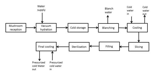
Fig 1.3: The block diagram of mushroom flow in canned mushroom production
