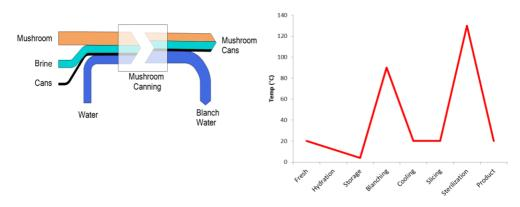
*Fig* 1.4: *Left*: Mass balance of canned mushroom production shown with Sankey diagram. *Right*: Temperature change in mushroom at various unit operations.
