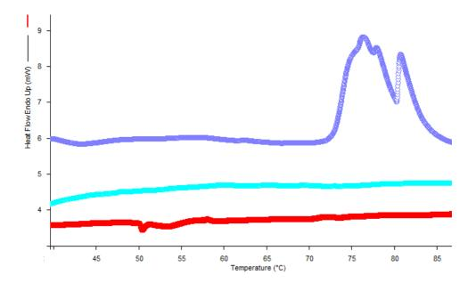
Fig 4.5: DSC curve of fresh (Top), milled (middle) and frozen (bottom) samples.
